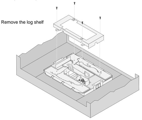
**NOTE**: The grate is not shown in the illustrations to better show component removal. It may be left in place during accent light installation.
